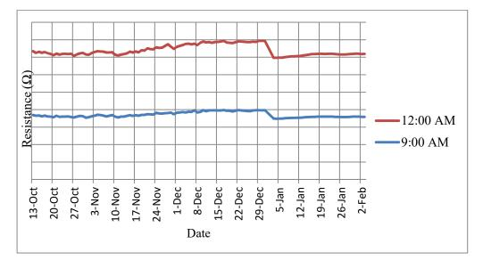
Figure 4.1: Date and temperature dependence of resistance graph
